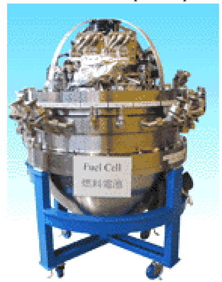
The fuel cell container is shown below with the top cover opened
