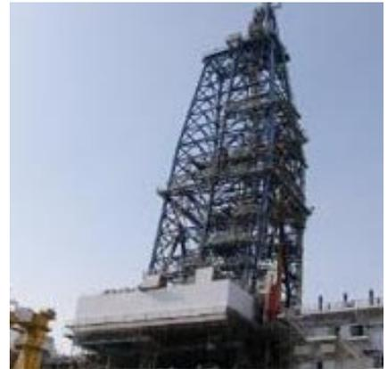
*Derrick: Height 70.1m x Width x 18.3m x Length 21.9m x Hanging Capacity: 1,250ton*
