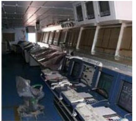
*The bridge includes a series of control equipment for vessel movement (engine and ballast control, control console for the DPS, the acoustic positioning system, etc.)*
