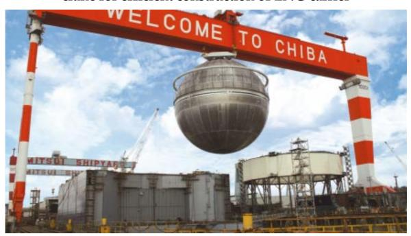
Mitsui Engineering & Shipbuilding Co., Ltd. recently installed a spherical LNG tank as an integrated unit onto the LNG carrier under construction at its Chiba Works. A 1,000-ton capacity gantry crane was used for the installation. A spherical LNG tank weighs about 700 tons as fabricated for the 145,000m³ LNG carrier (Moss type LNG carrier).
