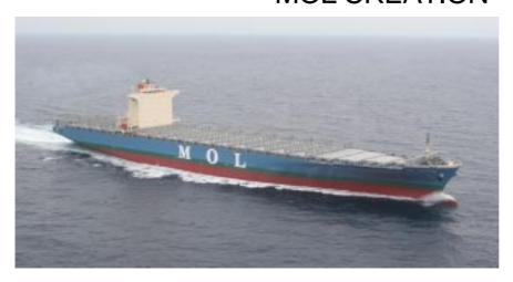
Mitsubishi Heavy Industries, Ltd. (MHI) has completed construction of the MOL CREATION (HN: 2225), a large container carrier capable of carrying 8,110TEUs, for delivery to Mitsui O.S.K. Lines, Ltd. (MOL) at its Nagasaki Shipyard & Machinery Works.
