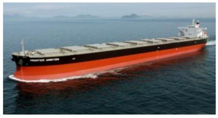
Principal particulars L (o.a.) x B x D x d: 288.93m x 45.00m x 24.70m x 18.15m DWT/GT: 180,253t / 90,092
