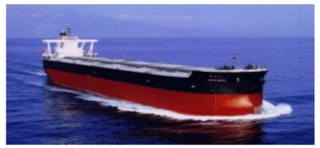
The 300,000DWT-type ore carrier, OITA MARU, was delivered to Kemp Maritime S. A. at the Tsu Shipyard of Universal Shipbuilding Corporation on Mar. 19, 2010. The OITA MARU is the 11th vessel of a new design series of the Unimax ore carrier, dedicated to transport of iron ore from Brazil to Japan.
