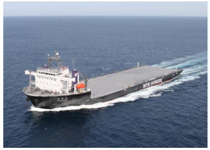
Mitsubishi Heavy Industries, Ltd. (MHI) has completed construction of YAMATAI, a module carrier with the designed module carrying capacity of 3,000 tons x 2 units, for NYK-Hinode Line, Ltd. This is the first of two sister vessels built at the Nagasaki Shipyard & Machinery Works.
