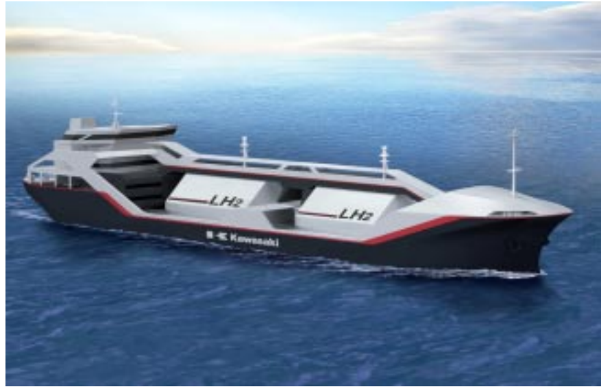
An appearance of the LH2 carrier (2,500m 3 capacity)
