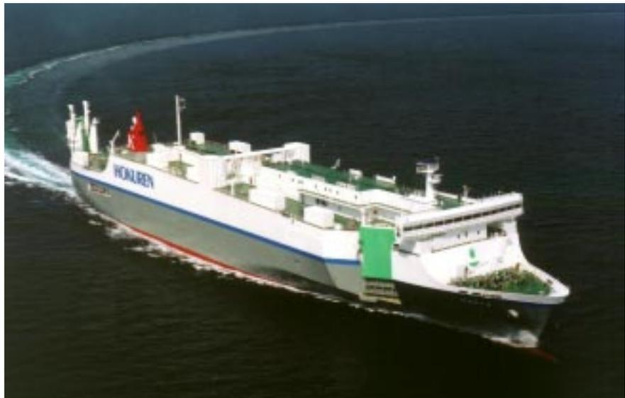
has become easier with one bow thruster and two stern thrusters. These thrusters use controllable pitch propellers and can be operated at the starboard side of the wheelhouse bridge, where the operation console and joystick system are installed. The joystick allows one man control of the main engine, bow, and stern thrusters.
