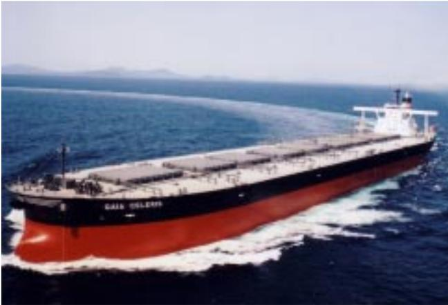
The GAIA CELERIS has the strengthened hull like a double hull construction to cope with transport of a variety of cargo ores. The vessel has five cargo holds and nine hatches, and the cargo holds are designed to be suitable for cargo handling and carriage of iron ore.
