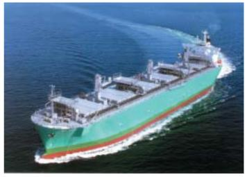
Cargo hold capacity: 102,040m<sup>3</sup>  $(grain), (3,603,542 ft^3)$ Main engine: MAN B&W 6S 50 MC-C diesel x 1 unit
