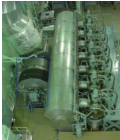
Main engine (Hybrid turbocharger seen in the blue square line)
