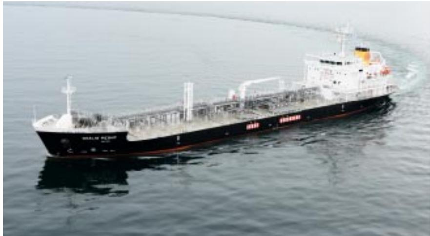
performance in ship speed and uses the super VecTwin rudders and bow thrusters. The hull form design and equipment have improved lateral movement and turning on the spot, increasing the maneuverability compared to before.
