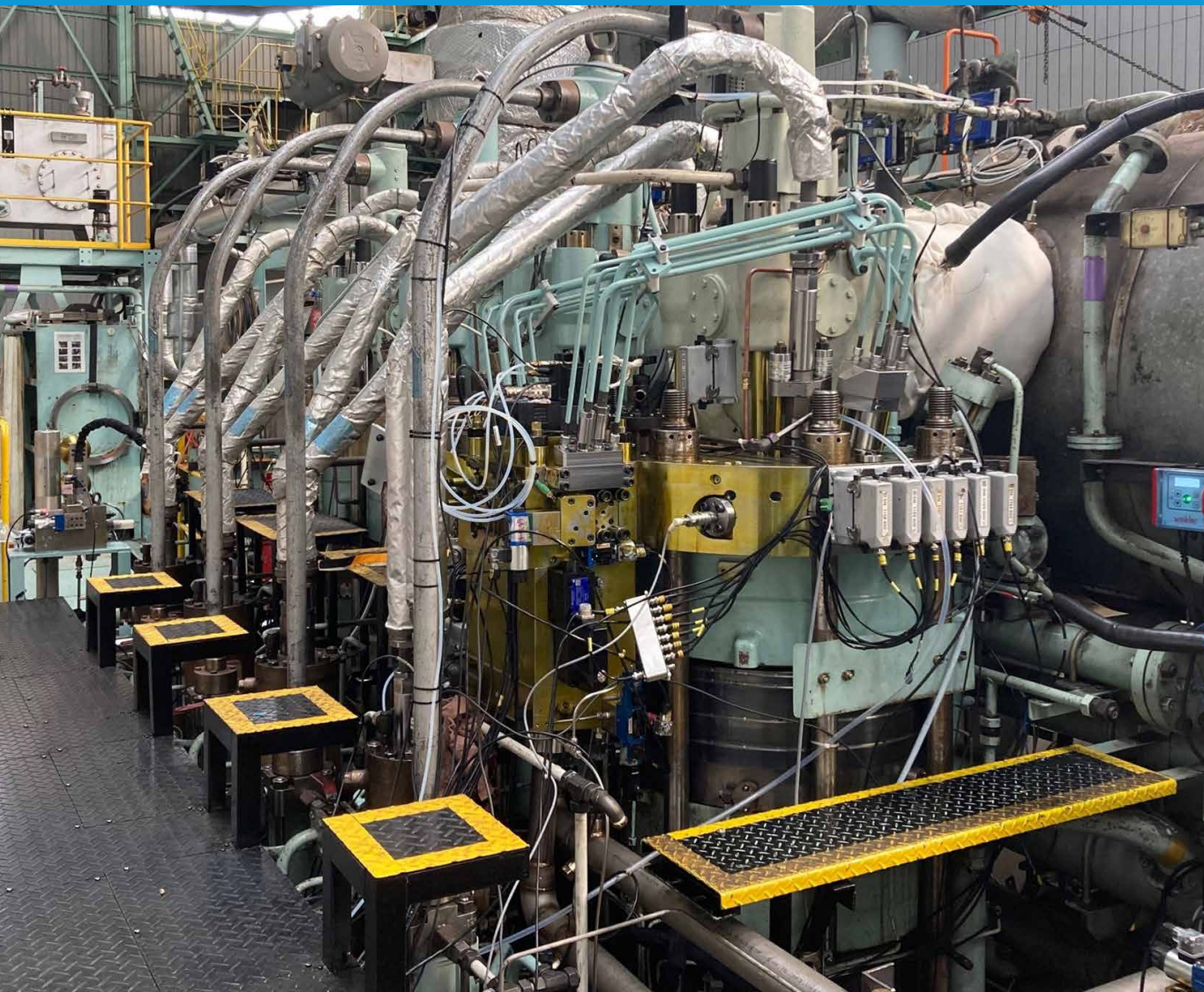
Hydrogen combustion test on 4S50ME-T
