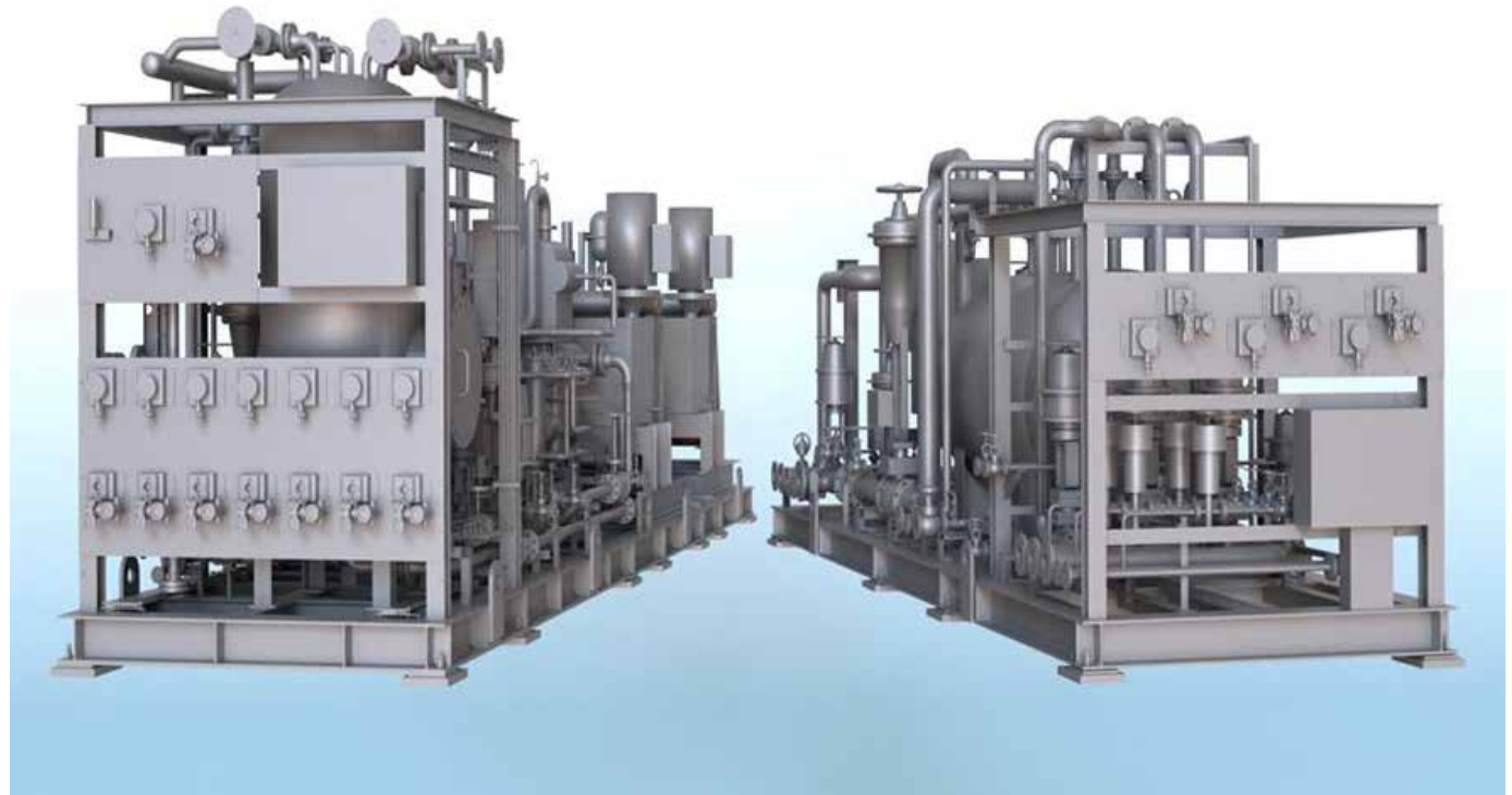
Ammonia Fuel Supply System (High-pressure and Low-pressure AFSS module)
