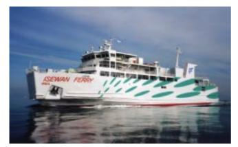
include the bow and stern ramp doors provided at the level of the car deck that can accommodate buses, trucks, and passenger cars. The passenger cabins are arranged on the promenade and cabin decks. The sunroom is positioned at the stern behind the special room. Large square windows are fitted to provide brightness and amenity. Barrier-free measures are fully considered for elderly and disabled passengers.
