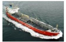
Owner: Panther Navigation Inc. Builder: Shin Kurushima Dockyard Co., Ltd. Hull No.: 5317 Ship type: Chemical tanker L (o.a.) x B x D x d (summer): 159.98m x 26.8m x 14.2m x 9.876m DWT/GT: 25,435t/16,232t Main engine: 6UEC52LA diesel x 1 unit Speed, service: about 15.5kt Classification: NK Completion: Mar. 9, 2005
