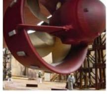
Side thruster at the bow of the vessel 2550kW x1
