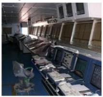
The bridge includes a series of control equipment for vessel movement (engine and ballast control, control console for the DPS, the acoustic positioning system, etc.)
