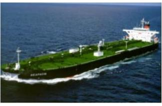
diesel x 1 unit Output: 12,240 kW x 105.0rpm Speed, trial max.: 15.35kt Ship type: Crude oil carrier Classification: ABS Completion Sept. 9, 2005
