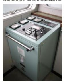
cient rudder are controlled integrally by using the joystick and rotation dial. Therefore, it became easy and simple to control the ship's motion (surging, swaying and yawing) accurately. This system enables easy berthing operation and helps to avoid the associated rick
