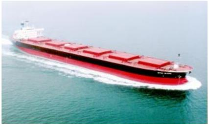
by the gravity system can be demonstrated for shortened deballasting time to cope with the high-speed loading facilities at ports. As one of the measures for loading iron ore, special coating is applied to the hold surfaces for improved maintenance. The vessel is equipped with necessary outfittings and arrangements together with required devices to enter cargo-unloading berths in Japan.
