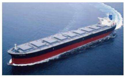
Ballasting and deballasting work can be efficiently achieved by separation of the topside tank and bottom side tank. Ballast water can be changed during navigation for protection of the marine environment
