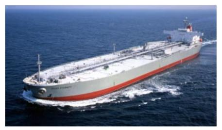
Sumitomo Heavy Industries Marine & Engineering Co., Ltd. (SHI-ME) has delivered the 105,000 MTDW double-hull Aframax clean petroleum product carrier RIVER ETERNITY to Wealth Line Inc. at the SHI-ME Yokosuka Shipyard. The vessel was designed to carry clean petroleum products such as naphtha, jet fuel, gasoline, diesel oil, fuel oil and gas oil.
