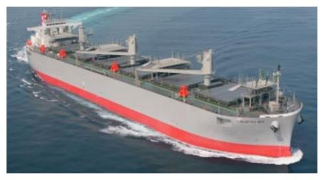
to improvement of speed performance in rough weather conditions (about 5% power saving compared with the ordinary bulbous bow). The Flipper Fins, a set of fins of the simplest structure, is used to improve propulsive efficiency for fuel oil saving.
