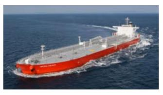
B (mld.): 42.00m D (mld.): 21.50m d (mld): 15.62m (summer, full load) DWT/GT: 115,577t/59,164 Cargo tank capacity: 126,606m³ Main engine: Mitsui B&W 6S60MC-C diesel x 1 unit MCR: 11,700kW x 95.0 min¹
