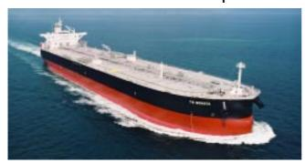
Tsuneishi Holdings Corporation completed the 107,500DWT type Aframax size crude oil tanker, TH SONATA on Oct. 2, 2008. The vessel complies with the new regulation of IACS Joint Tanker Project Common Structural Rules for Double Hull Oil Tankers (except performance standard for protective coatings for ballast tanks).
