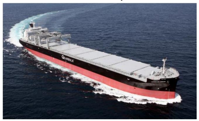
Oshima Shipbuilding Co., Ltd. delivered the 72,863DWT CORELLA ARROW, the world's largest open-hatch bulk carrier for general cargoes, to Glory Ocean Shipping S.A. in May 2009.
