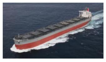
Hull No.: 1635 Ship type: **Bulk carrier** Length, o.a.: 292.00m Length, b.p.: 288.00m Breadth, mld.: 45.00m Depth, mld.: 24.70m Draught, mld.: 18.20m (full load, summer) DWT/GT: 182,718t/92,977 Main engine: Kawasaki-MAN B&W 6S70MC-C (Mk7) diesel x 1 unit
