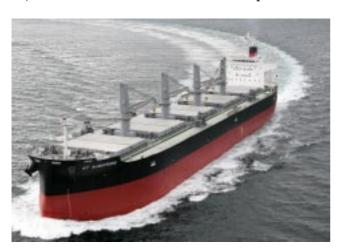
The bulk carrier is the flush deck type with a forecastle and has five cargo holds that can load a variety of cargoes such as cereals, coal, ore, steel products, etc. Four deck cranes installed between hatch covers on the ship centerline facilitate cargo han-
