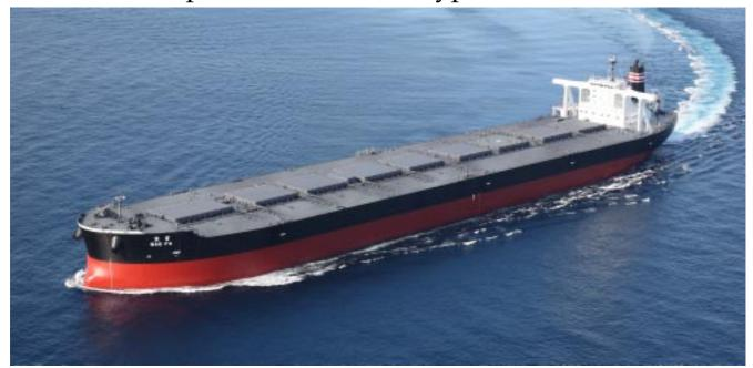
Namura Shipbuilding Co., Ltd. delivered BAO FU, a 250,877DWT ore carrier, to Wealth Line Inc. at its Imari Shipyard & Works on Oct. 26, 2010. This is the first vessel of the 250,000DWT type of ore carrier and the principal dimensions of the vessel satisfy the restrictions of Port Hedland, Port Walcott, and Dampier, which are the three major ports in Western Australia, so this type is called WOZMAX (Western Australia [Aussie: OZ] Max).
