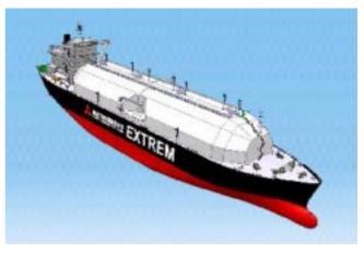
which achieves higher thermal efficiency through effective use of thermal energy by reheating steam. Together with downsizing, weight reduction and hull lines improvement, the new ship achieves a substantial 20% reduction in fuel consumption compared to conventional ships.
