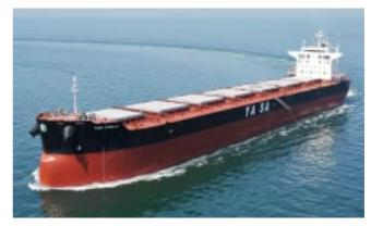
L (o.a.) x L (b.p.) x B x D x d: 229.00m x 224.00m x 32.24m x 20.20m x 14.598m
