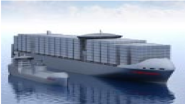
LNG-fueled containership and fuel supply barge
