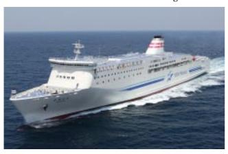
The vessel is equipped with the CRP POD system, which achieves an extremely low fuel consumption compared with ordinary RoPax ferries. In addition, this vessel also has a steam turbine generator as a waste heat recovery system so that additional energy saving can be achieved. The passenger facilities of this vessel are de-
