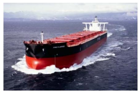
bow above the waterline uses the Ax-Bow design that can decrease added wave resistance at sea. Deck machinery such as windlasses and mooring winches and hatch covers are driven by an electric-motor system for oil leak prevention on the deck.
