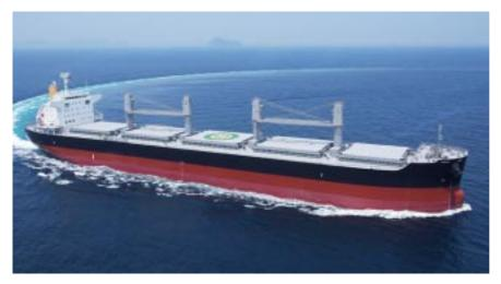
61,000DWT-type bulk carrier "IS" I-STAR
