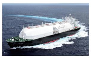
the tanks with an integrated cover, which makes such supporting structures unnecessary, the new design also improves maintainability.
