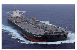
While the optimization of deadweight and cargo tank capacity under such restrictions, the vessel is extended in full length and refined on lower resistance hull form with state-of- the-art comprehensive technologies to achieve drastic decrease of fuel oil consumption. Besides that, her hull performance is sophisticated with optimized energy-saving devices, such as Semicircular Duct and Surf-Bulb (Rudder
