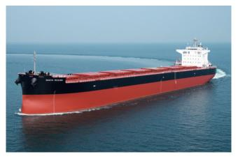
$\begin{array}{c} \mbox{Hull No.:} & 1329 \\ \mbox{L (o.a.) x B x D x d: 229.00m x 32.24m} \\ \mbox{x 20.20m x 14.668m} \end{array}$
