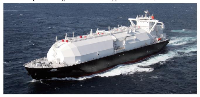
Mitsubishi Heavy Industries, Ltd. (MHI) completed construction of the LNG VENUS (HN:2295), a new generation MOSS-type LNGC "SAYAENDO" with a tank capacity of 155,691m³ (100% full), and delivered the vessel to Osaka Gas International Transport Inc. and Mitsui O.S.K. Lines, Ltd. at the Nagasaki Shipyard & Machinery Works on November 13, 2014.
