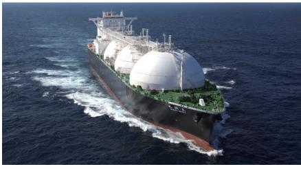
riers. The ship features a fully optimized hull structure for reduced weight, as well as a hull shape that is optimized for the maximum propulsive performance. Furthermore, Kawasaki Advanced Reheat Turbine Plant, which is proven to substantially improve transport efficiency, is adopted as the main engine.
