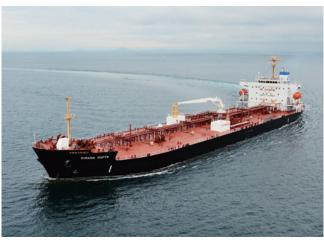
The tanker is a wide beam and shallow draught type with the navigation draught limited to 7.13m. The cargo tanks including slop tanks are segregated into 12 sections. These compartments are protected by double side-shells and bottom to prevent outflow of petroleum products to avoid marine contamination. Fuel oil tanks are also designed with double-skin
