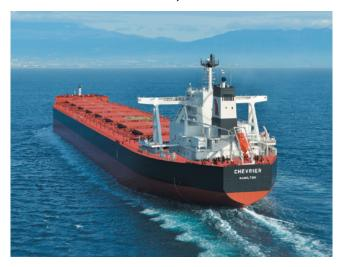
DWT/GT: 182,625t/93,297 Main engine: MAN B&W 7S65ME-C8.2 diesel x 1 unit
