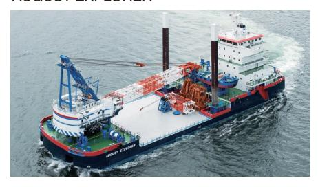
rials such as artificial fishery-reef blocks and construction blocks. A remotely operated vehicle (ROV), unmanned survey helicopter, and research-lab container booth can be loaded for investigation purpose.
