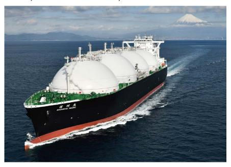
decrease overall ship weight, enhanced the hull-shape design, and adopted a two-motor, twin-screw propulsion system to achieve the optimum propulsive performance, and has integrated a DFD\* electric propulsion system which increases fuel efficiency at all speeds.
