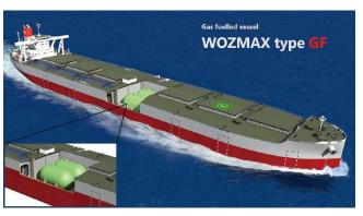
(3)The vessel has enough cruising capacity to make the round-trip between Singapore and Brazil in only gas-fuel mode without refueling.
