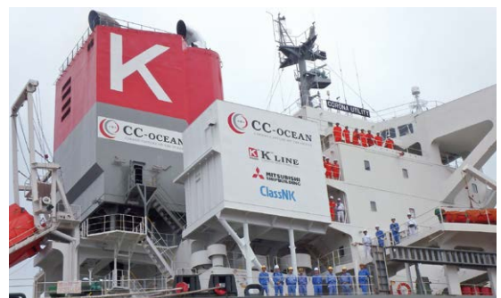
Marine-based CO 2 Capture System installed on board the CORONA UTILITY
