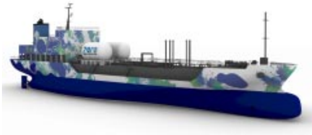
Image of this ship with the concept of arranging the hydrogen fueled engine as a power generator in the engine room for electric propulsion
