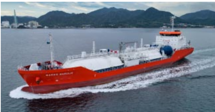
Photo shows Japan's first LPG-powered small-scale LPG carrier built by Sasaki Shipbuilding, which will pioneer the next generation of alternative-fueled small ships
